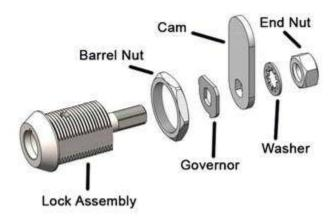
Insert the lock assembly through the original hole.
